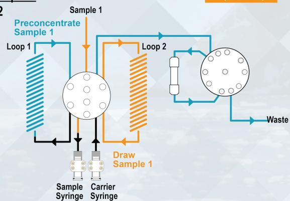
To maintain 100% duty cycle for sample loading and enable the automated processing of large samples, a dual loop configuration is used:
